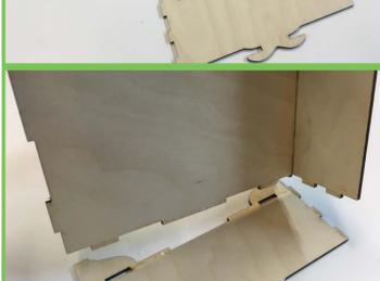
Gluing in assembly to the box front. Zooming in shows good placement of glue.
