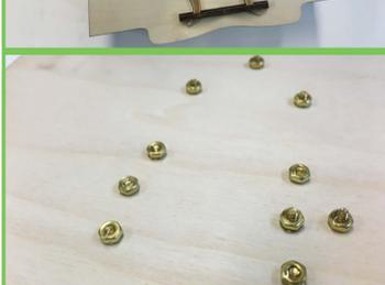
Place the washers and nuts on the back of the lid and tighten down snugly. This should seat the screw heads into the wood. Then loosen the nuts 1/8 turn to prevent binding. Set aside the lid.
