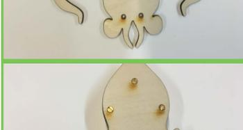
Note the backpiece has holes with indentations on one side. This side will face up.
