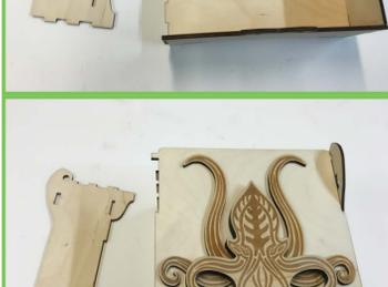
Get the lid and slide it into the right hinge and drop it onto the front tab.
